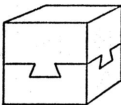
We show an isometric view of two wood blocks that have been dove-tailed together. The other three faces look just the same as the three shown. How was the cube constructed?
